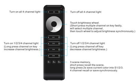
Note: RS6 match with 4 channel receiver only, such as V4, each channel connect with one single color LED strip.
